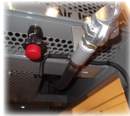
Figure 14: Engine throttle control and Air inlet connection
