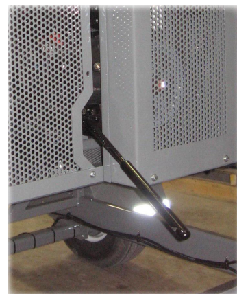
Figure 30: Clutch handle and operating lever
