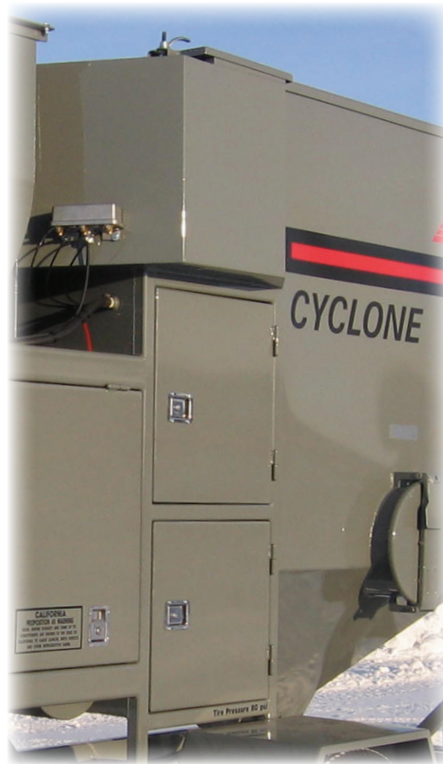
Figure 9: HEPA filter on top, storage compartments below
