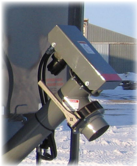
Figure 10: Rear discharge auger butterfly valve lever
